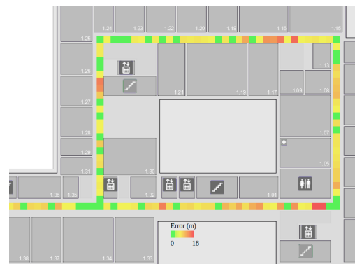
Fig. 9: Spatial distribution of WiFi fingerprinting based location estimation errors on the floor plan.
